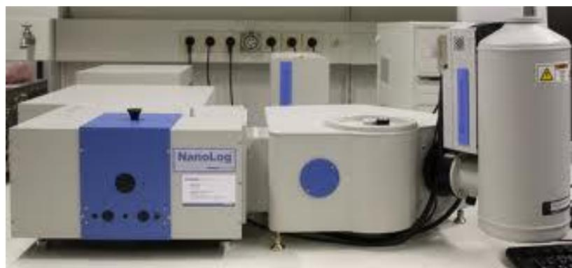
*Slika 3.19.* Horiba Jobin Yvon Fluorolog FL3-22 spektrofluorometar
